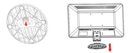
3. Press the release button on the stand while pulling away from the monitor.
